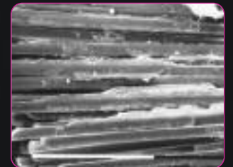
ENA POST sections under magnification (by Prof. V. Kaitzas).
